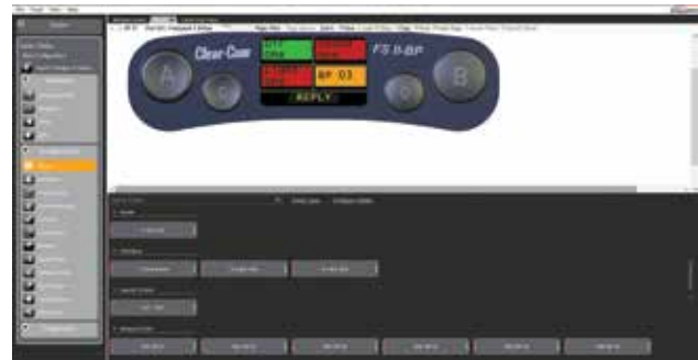
FreeSpeak II Beltpacks are configured within the EHX (Eclipse HX Configuration Software). They benefit from all the features within the Eclipse HX matrix system.
